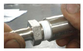
Insert into female fitting, make sure thread is located properly and tighten until sealed. Be careful not to wind the fitting back at all, as the tape is a 'one shot deal' and if you undo it it may not seal properly and you will have to re-tape it.
